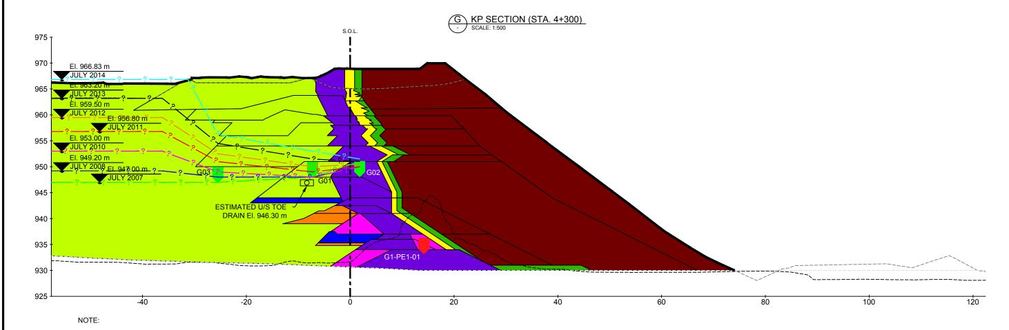
PIEZOMETER G1-PE1-01 STOPPED READING IN 2002 & G03 STOPPED READING IN MAY 2014.
