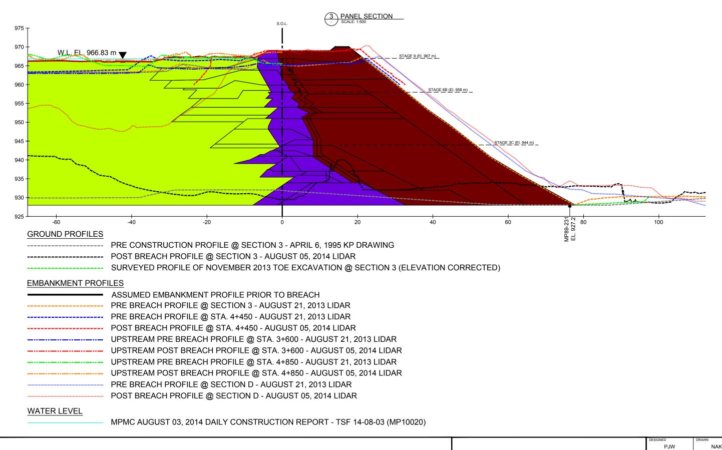
BASIS FOR GEOMETRY USED FOR STABILITY ANALYSIS
