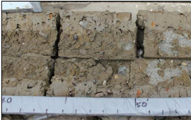
FIGURE D6.4.2A: UPPER TILL DESICCATED CRUST
