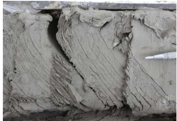
FIGURE D6.4.3B: UPPER GLU WITHIN BREACH AREA
