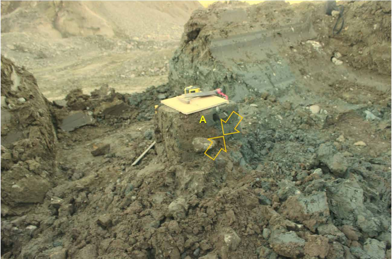
FIGURE 5: PHOTO SHOWING THE PARTIALLY TRIMMED BLOCK SAMPLE 2
