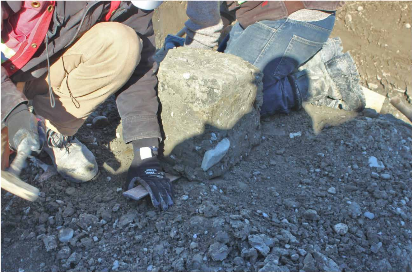
FIGURE 3: CHISELING THE BASE OF BLOCK SAMPLE 1
