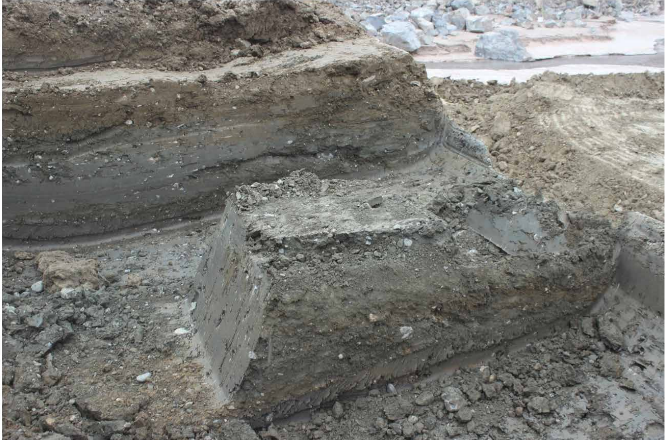
FIGURE 1: EXCAVATED PEDESTAL FOR BLOCK SAMPLE 1
