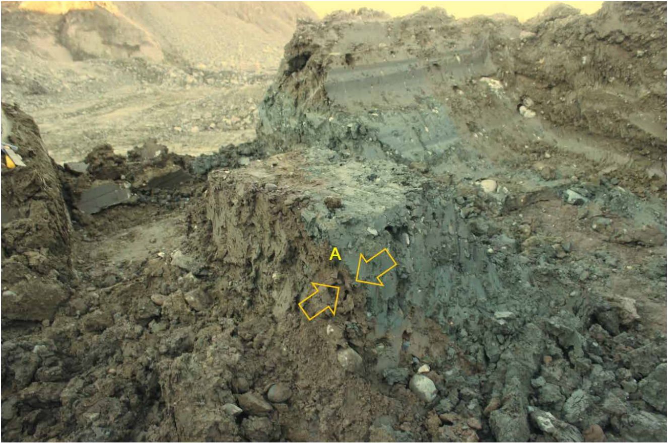
FIGURE 4: PEDESTAL FOR BLOCK SAMPLE 2
