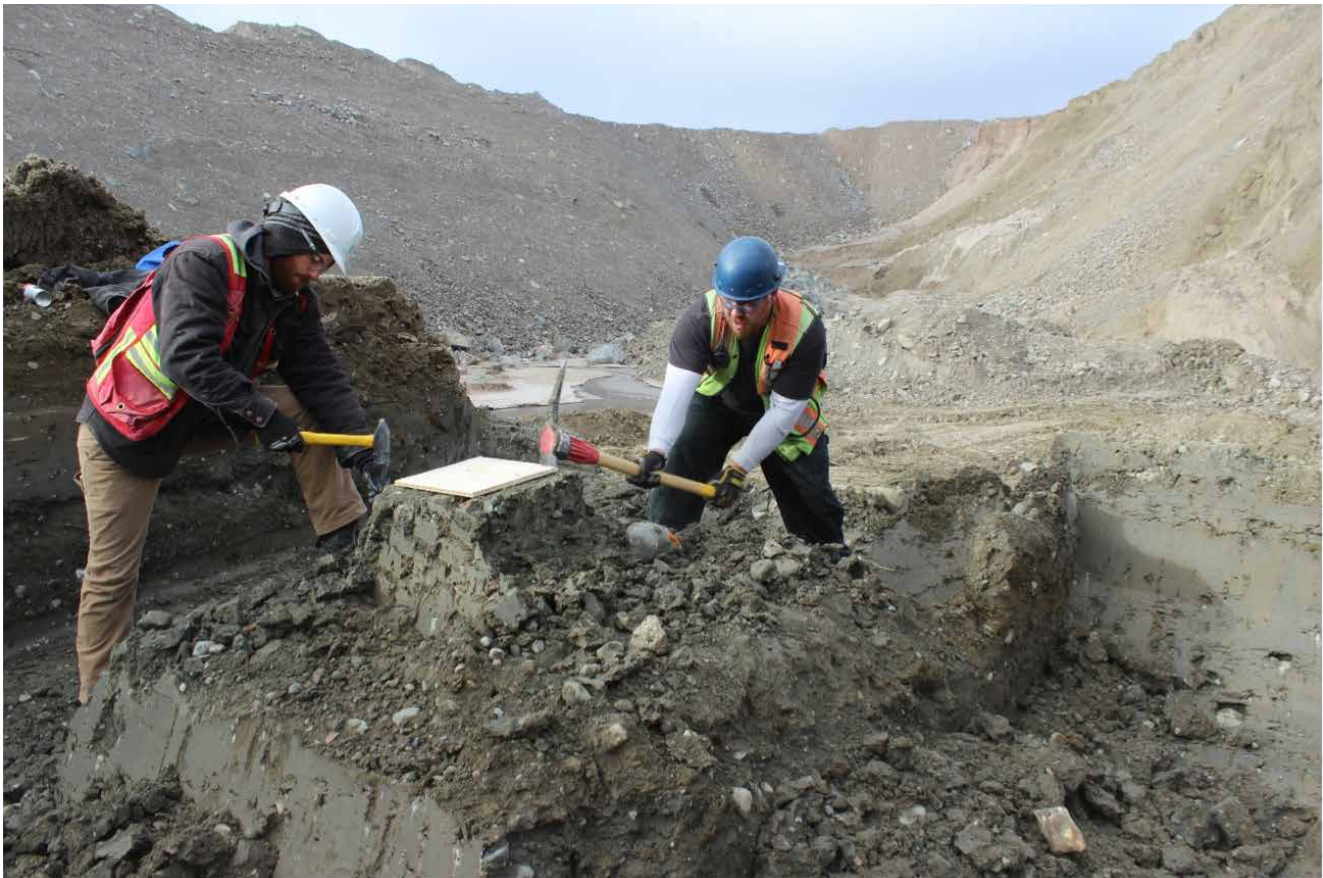
FIGURE 2: TRIMMING BLOCK SAMPLE 1
