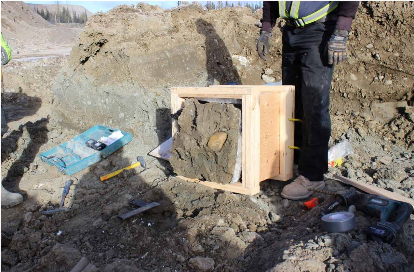
FIGURE 6: BASE OF BLOCK SAMPLE 2 READY FOR FINAL TRIMMING
