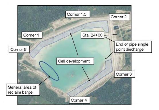
Figure 2.1: Tailings Discharge Plan
