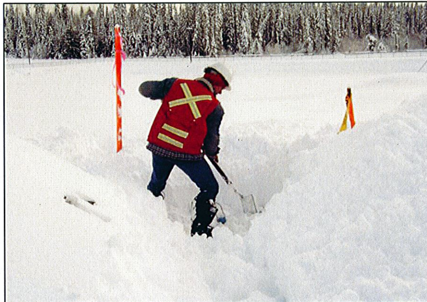
PHOTO 30 – Uncovering an inclinometer
