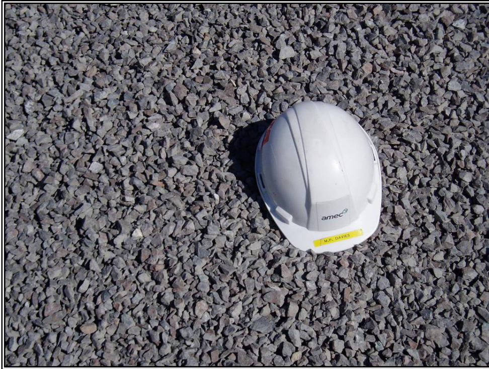
Photo 7: Main Embankment Transition Material
