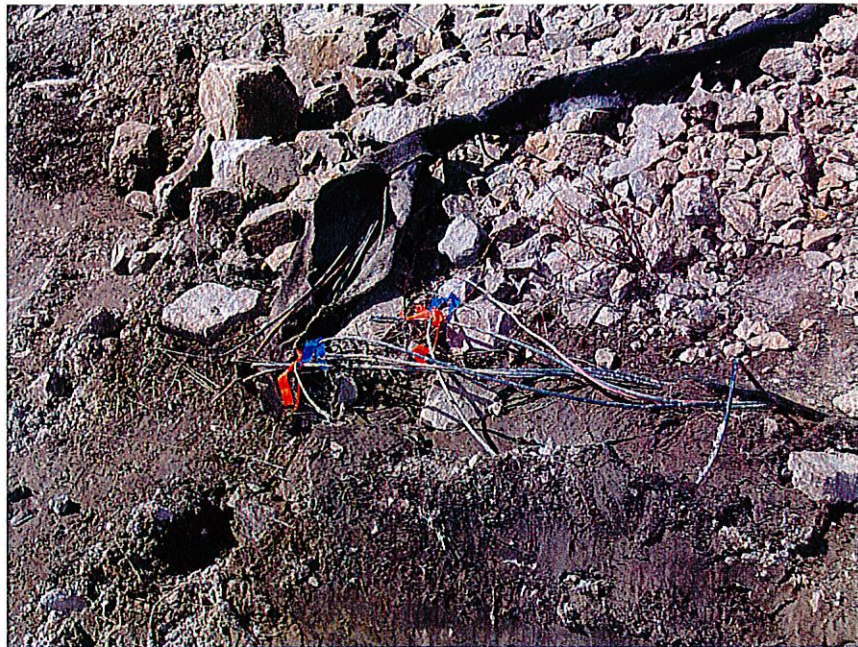
PHOTO 19: Damaged Piezometer cables at the Main Embankment.
