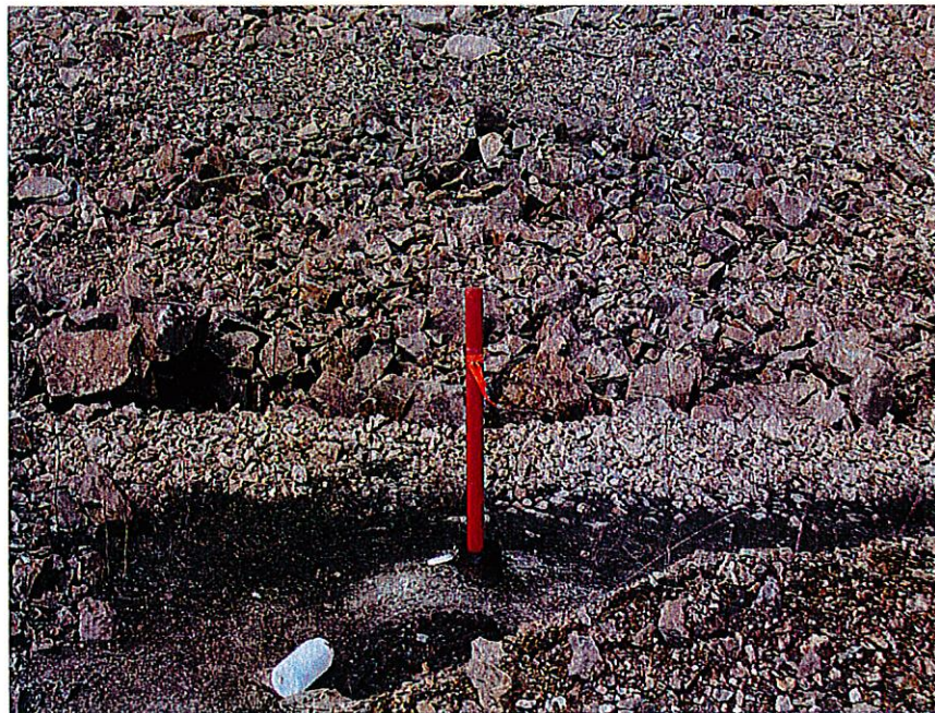
PHOTO 20: Existing inclinometers at the Main Embankment. These are to be extended during the Stage 5 Construction program.
