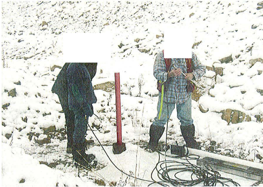
PHOTO 5 – Mount Polley personnel reading inclinometer.
