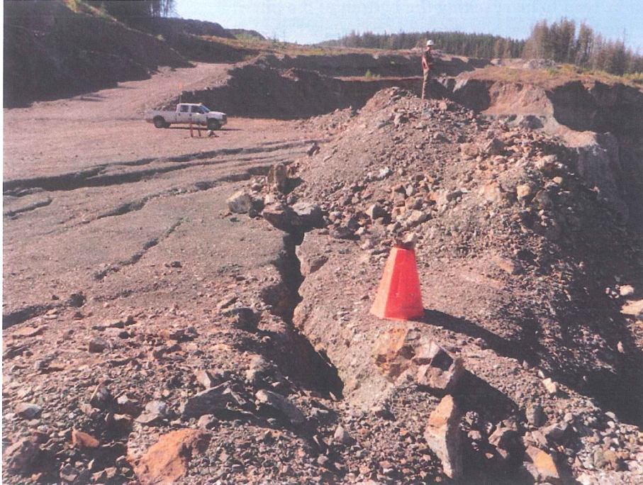
Photo 1: Tension Cracks and slump on south west crest of Wight Pit above underground access
