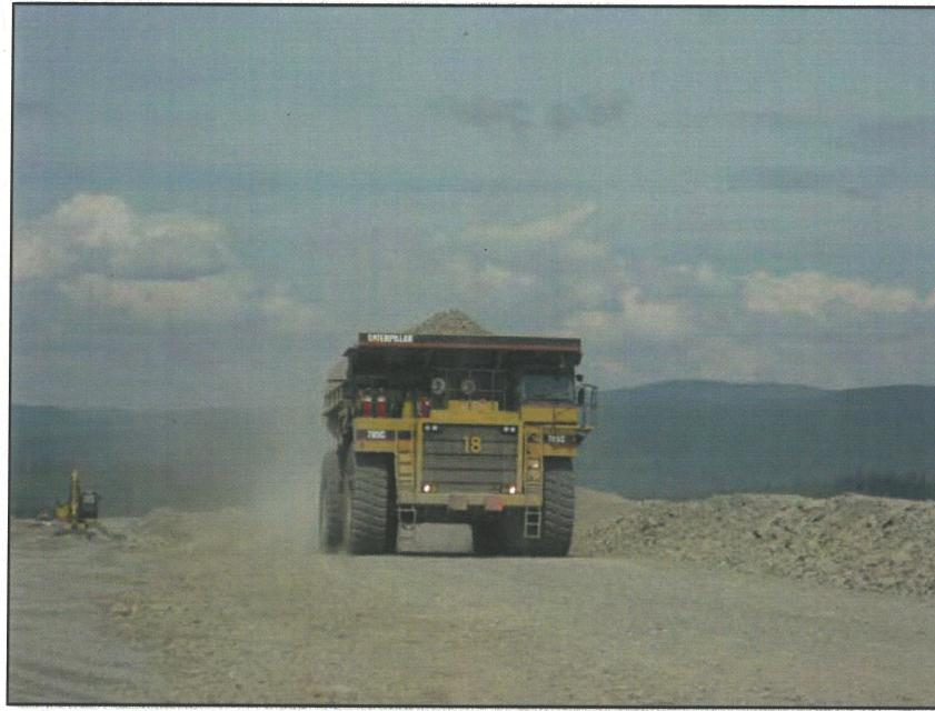
**PHOTO 14 – Zone C NAG waste rock hauled to the Main Embankment using the mine fleet**
