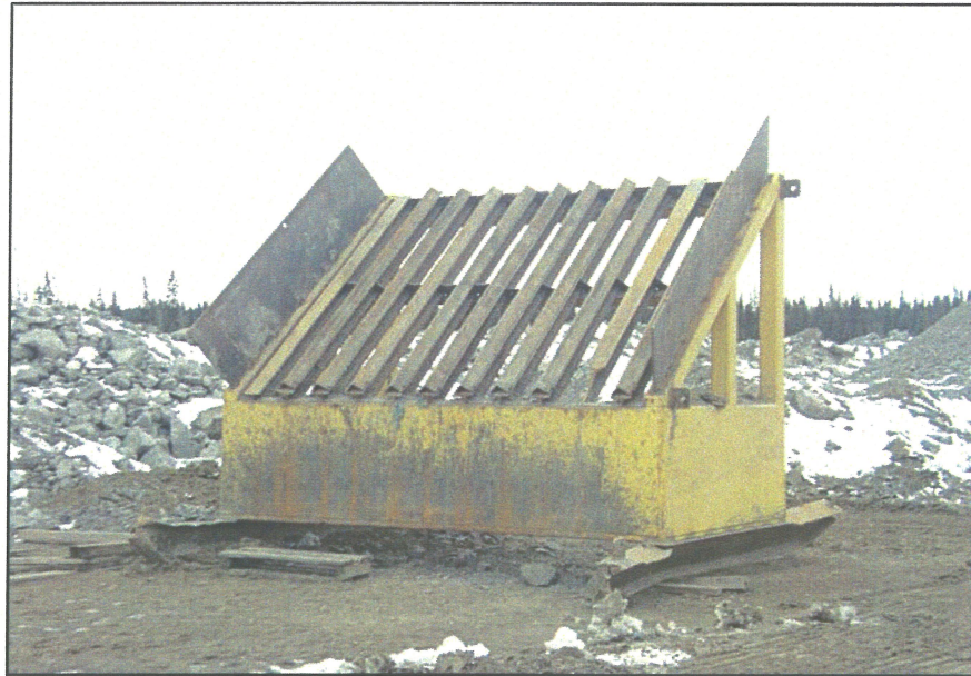
PHOTO 23 – Improved 'Grizzly' with sides to prevent Zone T material from spilling over
