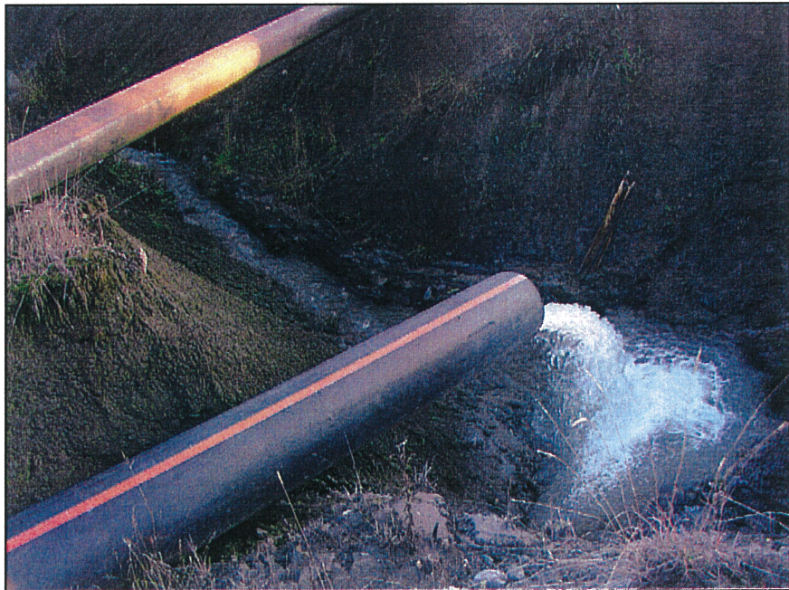
PHOTO # 8 – Tailings Discharge from M1 Dump Valve
