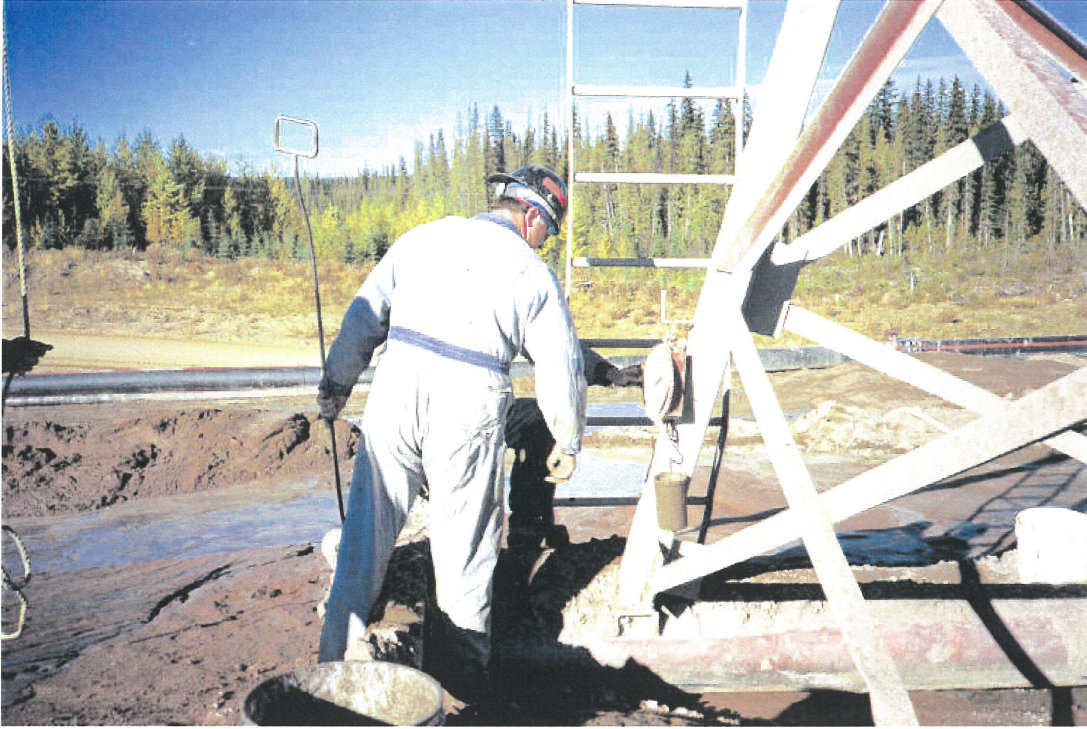
Photo No. 7: Upstream cycloned sand pulp density determination.
