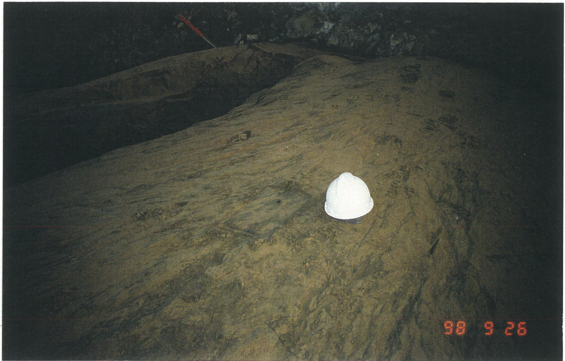
September 26, 1998 - Cycloned sand from trial program. Pile is fully drained, with slope 4H:1V. Sand produced from 50 inch cyclone. Sand dry density is 1650 \text{ kg/m}^3 at 8% moisture.
