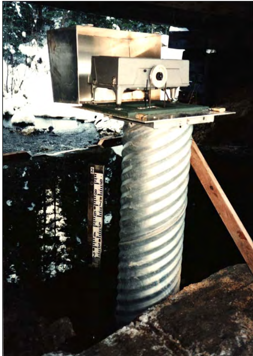
PHOTO 3 – Hazeltine Creek Gauging Station Chart Recorder and Original Staff Gauge. Photo taken in 1994. Notice that the gauge Height is ~0.200, and water level is ~0.1 m below weir crest
