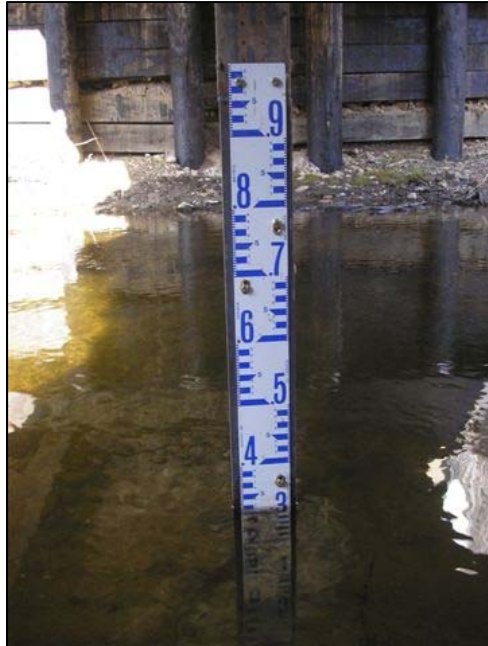
Photo 1: New Staff Gauge Installation, May 12, 2010.
