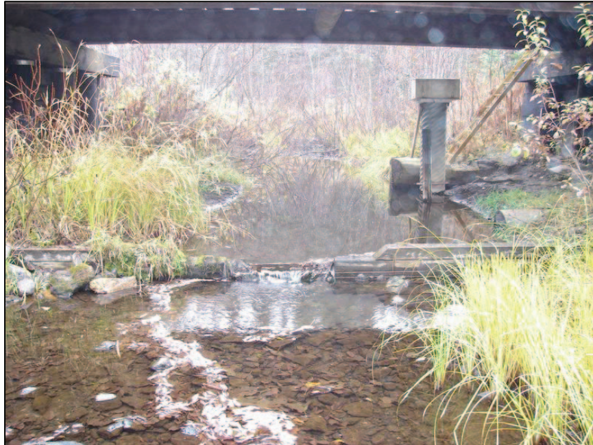
Photo 1 – Hazeltine Creek at hydrology station W7. Looking upstream at the stage recorder and weir.
