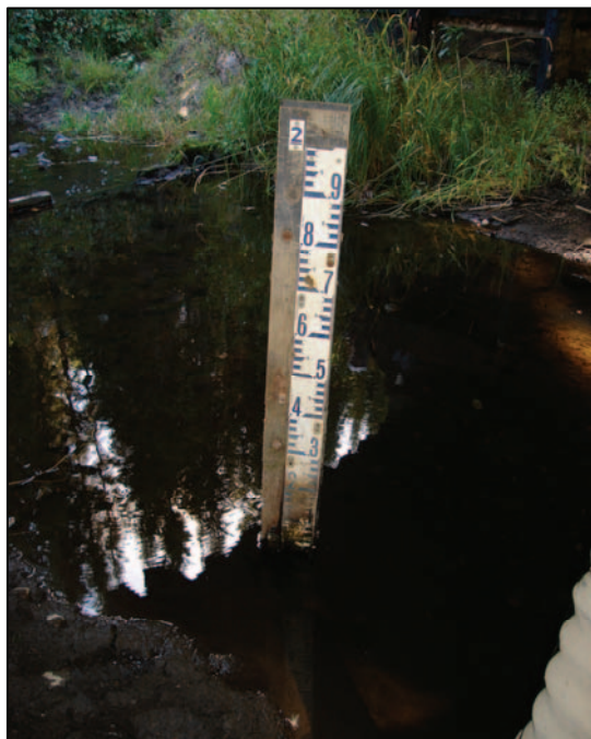
Photo 2 – Hazeltine Creek at hydrology station W7. Looking downstream at the staff gauge.
