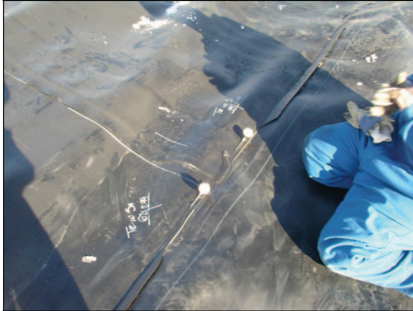
PHOTO 31 – Pressure testing a tie in seam
