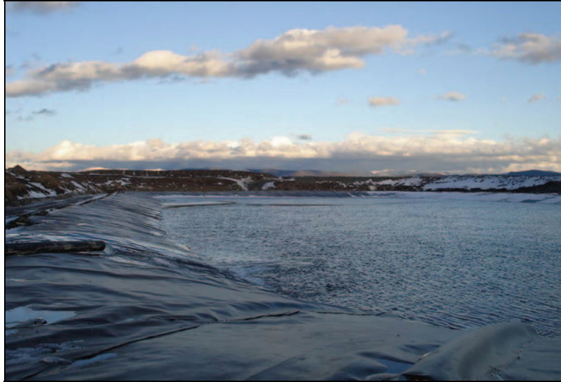
PHOTO 41 – Filling with water during hydrostatic test.
