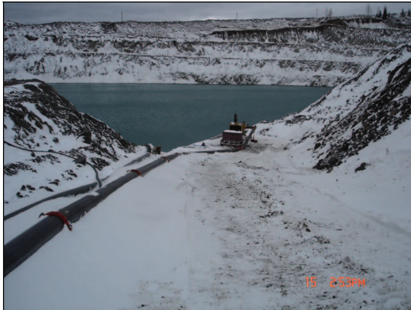
PHOTO 39 – Pump at the Cariboo Pit pumping to the leach pad.
