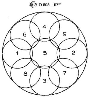
FIG. 4 Rammer Pattern for Compaction in 6 in. (152.4 mm) Mold
