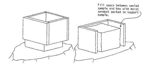
B. ENCASE EASILY DISTURBED SAMPLES IN BOX PRIOR TO CUTTING
