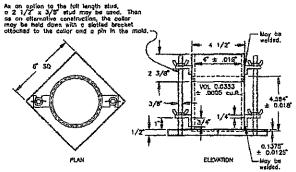
FIG. 1 4.0-in. Cylindrical Mold
