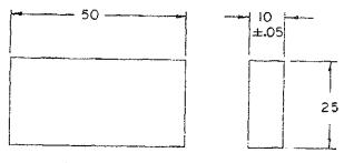
DIMENSIONS IN MILLIMETRES FIG. 4 Height-of-Drop Gauge
