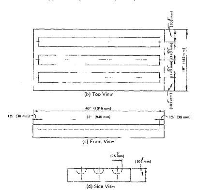
Non: 1—Top and bottom halves are identical. FIG. 3 Styrene Shipping Container for 3-in. (76-mm) Thin-Walled Tubes
