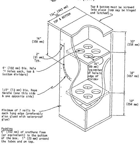
Material 3/4" (19 mm) thick plywood (exterior grade)
