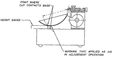
FIG. 2 Calibration for Height-of-Drop
