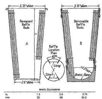
FIG. 2 Dispersion Cups of Apparatus
