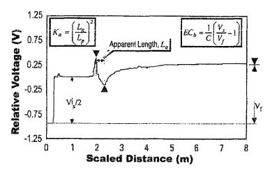
Figure 1. Typical TDR Waveform for Soil Showing Measurements to Obtain Apparent Dielectric Constant,  $K_a$ , and Bulk D.C. Electrical Conductivity.  $EC_b$
