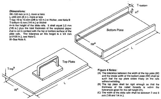
FIG. 5 Plastic Limit-Rolling Device
