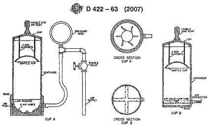
FIG. 3 Air-Jet Dispersion Cups of Apparatus 8
