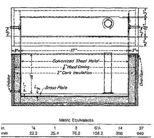
FIG. 4 Insulated Water Bath
