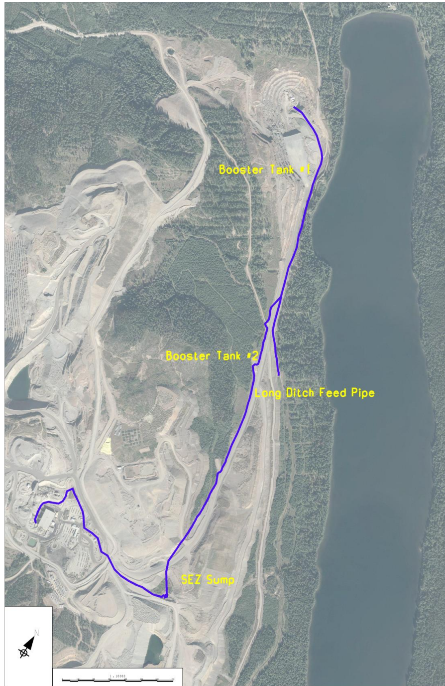
Figure 5.1.1.4.1 – Wight Pit Dewatering
