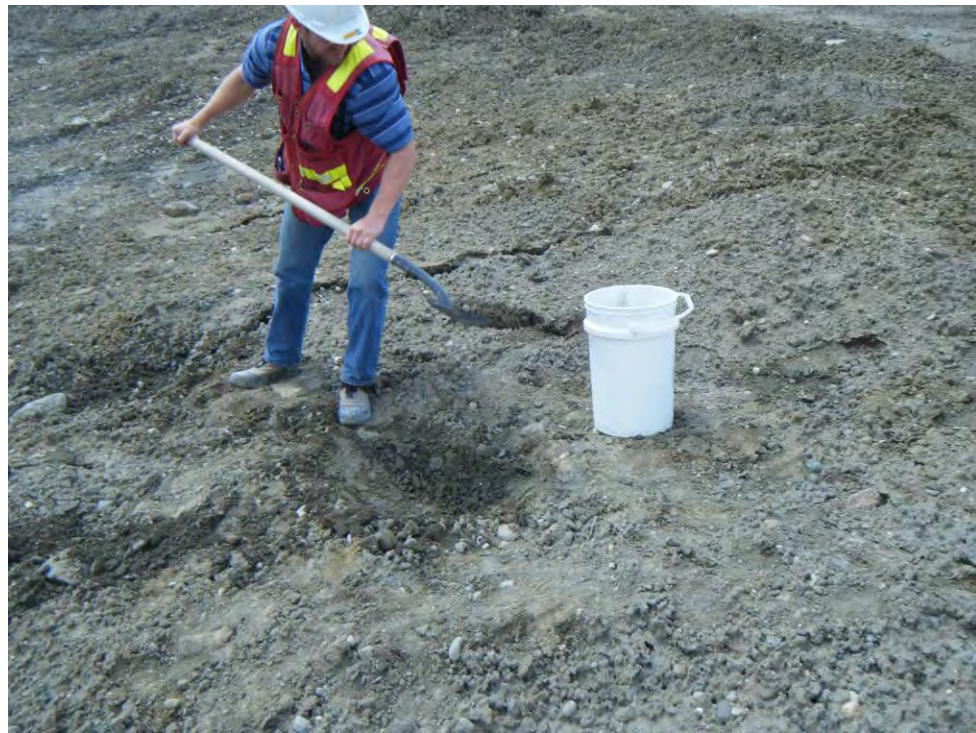
Photo 16: Surficial sampling of perimeter borrow pit.
