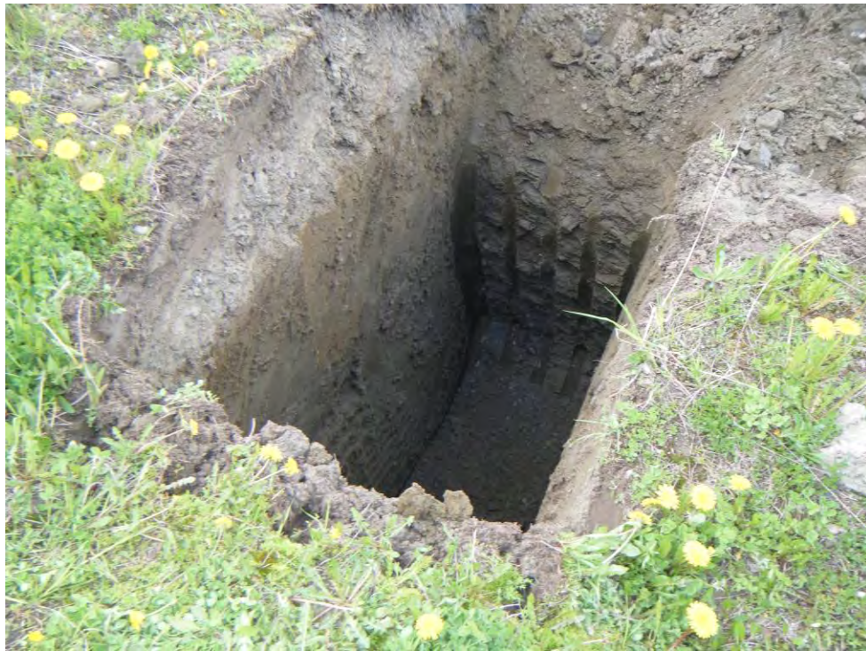
Photo 18: Test pits perform at the barge borrow pit.
