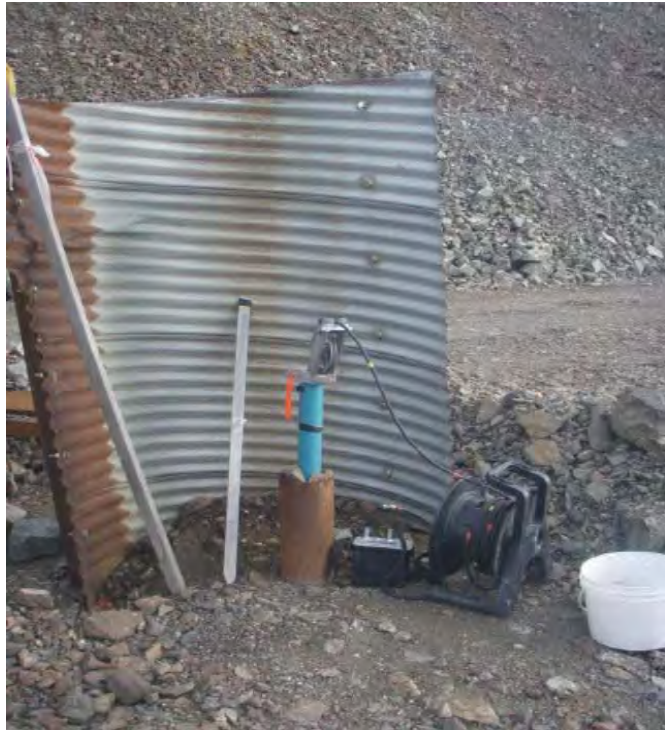
Photo 36: Slope Inclinator reading in progress.
