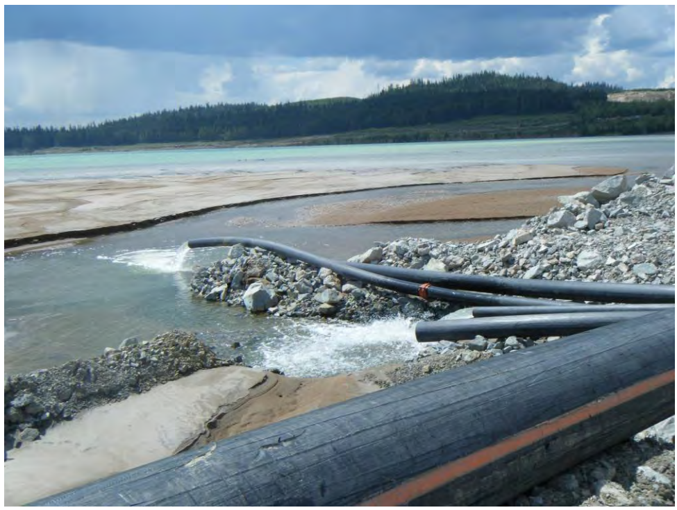
Photo 15: Perimeter seepage pond discharge into the TSF.
