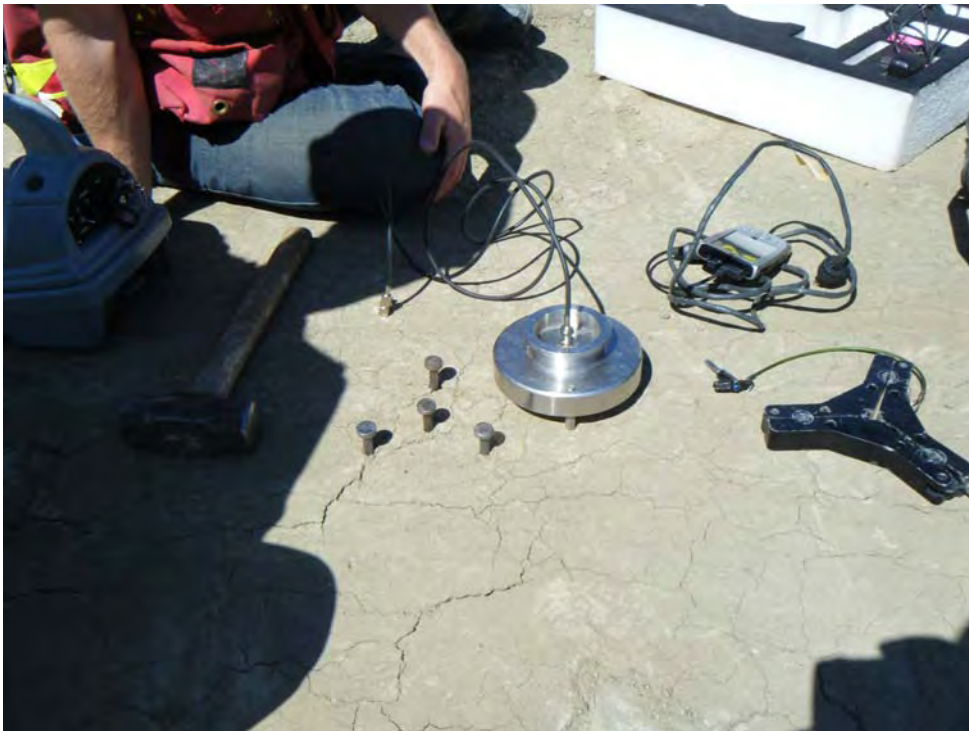
Photo 35: Compaction testing of Zone S, utilizing the MDI device.
