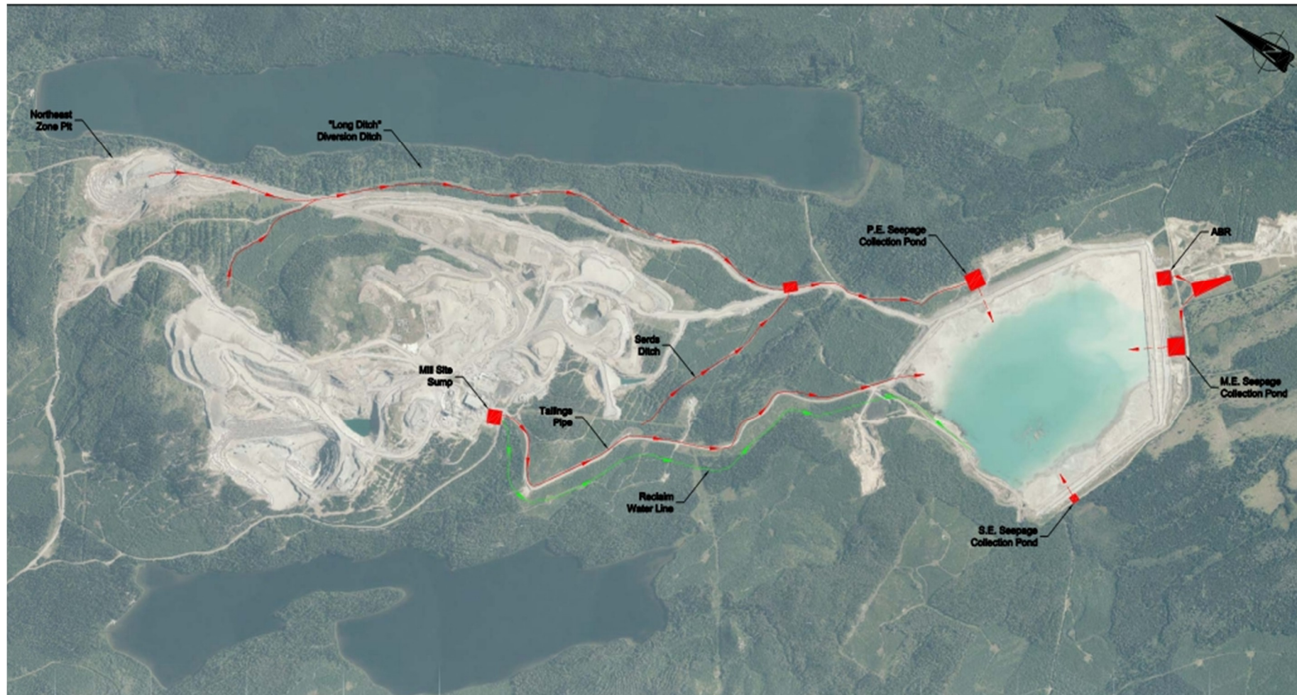
Figure 7.2 Site Water Management Schematic
