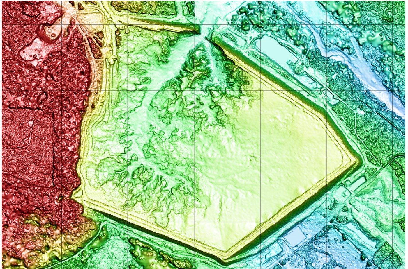
Mount Polley tailings dam topography after the breach
