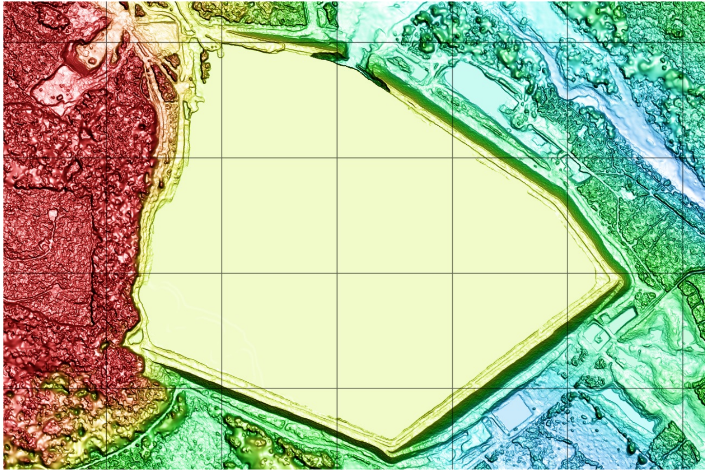
Mount Polley Tailings top surface a few days before the breach overlaid on the breached structure
