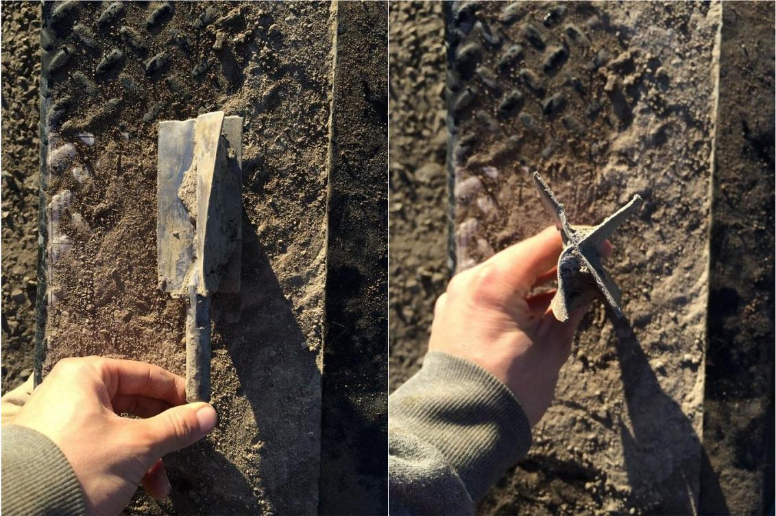
14-02091: Photos of the vane blade used for VST14-03 after consecutive tests at depths 12.2m, 12.5m, 12.8m and 13.13m.
