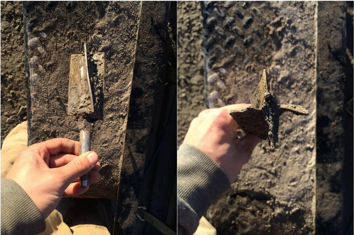
14-02091: Photos of the vane blade used for VST14-10 after consecutive tests at depths 11.78m and 12.08m.
